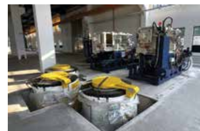
Multiple gravity casting stations have been installed in A-Forge's Vietnamese factory.
