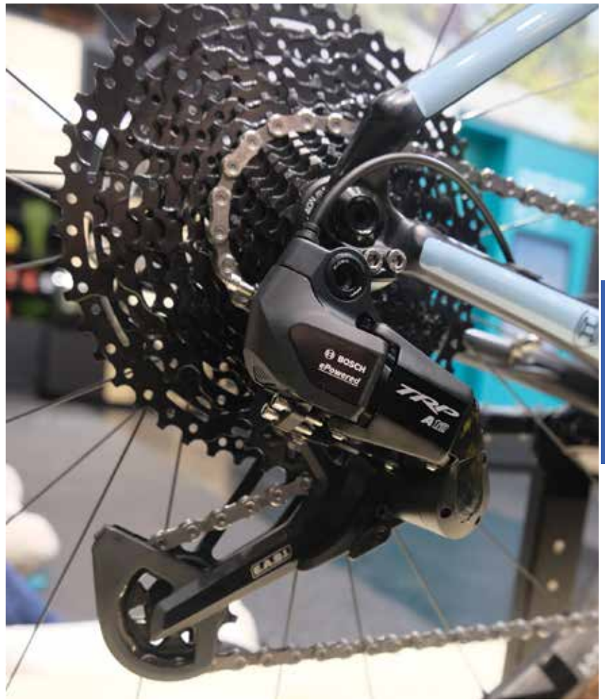
TRP's E.A.S.I. A12 drivetrain is the first 12-speed derailleur-based drivetrain to work with Bosch's eShift function.
