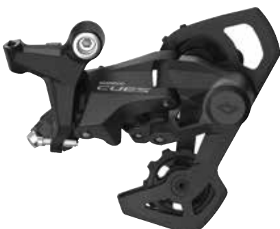
When opting for the shortest cage, Shimano's CUES derailleur offers plenty of ground clearance on kids' bikes.
