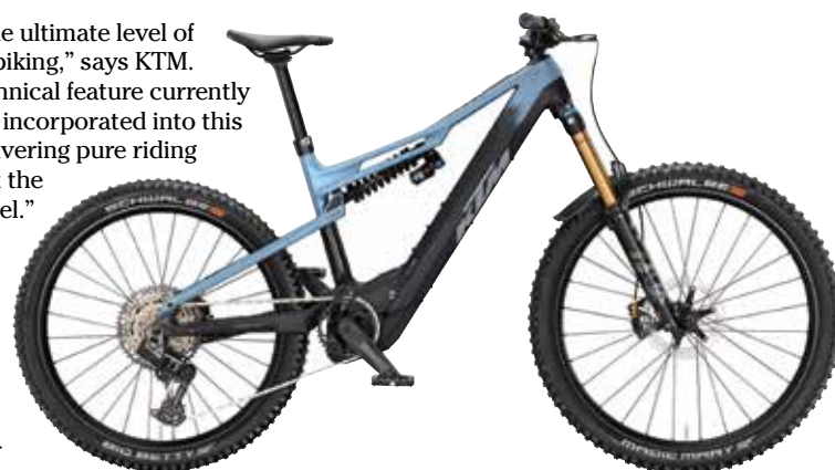
The Macina Prowler Prestige uses KTM's Power tube Top Loader for easy battery access.
