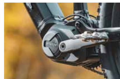
Ananda has designed the compact M230 mid-drive motor for use on eMTBs.
