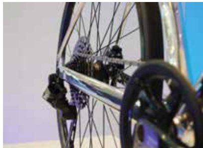
With the Q-Auto concept Shimano showed that its Di2 technology can provide automatic shifting on conventional bicycles.
