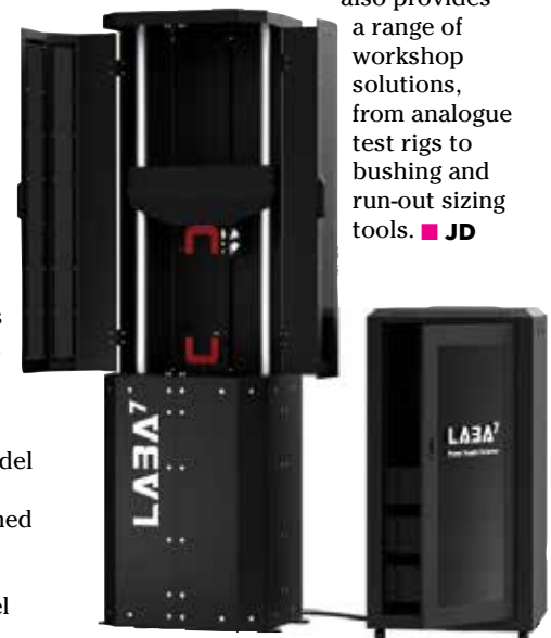
Grab data from your shocks with LABA's range of smart testing electromagnetic shock dynos
