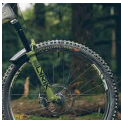
RockShox top-end aggressive forks will get an updated Charger 3.1 damper
