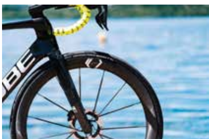
A minimalist number of aerodynamic carbon spokes characterise Newmen's latest Stream VONOA road wheels
