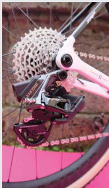
TRP's wireless and electronic Vistar derailleur premiers at Eurobike.
