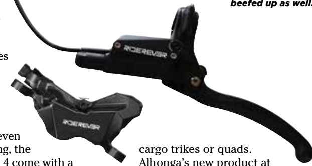
This four-piston caliper of Ride Rever has been adapted to work with 2.3 mm thick rotors, and the lever has been beefed up as well.
