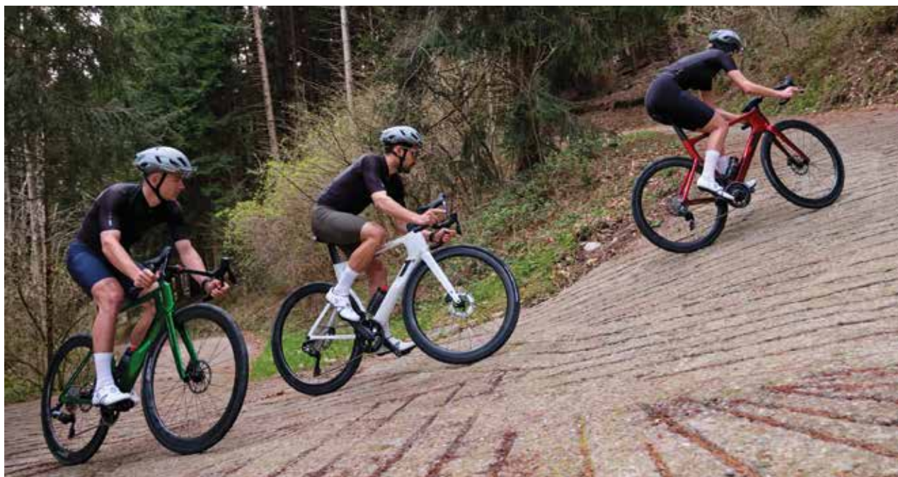
The Hi-Light frame is 3D-printed from grade 5 6Al/4V titanium
