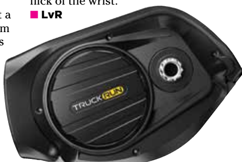
Truckrun's M12 is a seriously powerful mid-drive motor that cranks out up to 160 Nm of torque.
