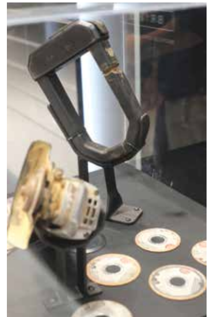
This Hiplok lock on display at Eurobike has been subject to 20 minutes of cutting
